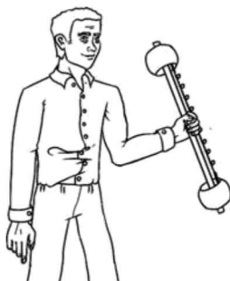
Fig. 14.1 A device for detecting the tidal effect of gravity. Two masses can slide along a rod, with a weak spring between them. A gravitational field will cause the geodesics to change in such a way that the two masses will approach or move away from one another, as the case may be. The extension or compression of the spring therefore indicates the tidal effect. [Image: Elsie Steane]
