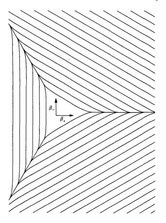
Some equipotentials,  $V(\beta) = \text{constant}$ , are shown for the function defined in equation (35). Equipotentials near the origin of the  $\beta$ -plane are closed curves for V < 1 and are omitted here.
