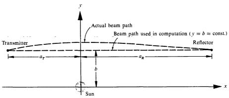
Figure 40.3. Diagram, in the PPN coordinate system, for the calculation of the relativistic time delay.
