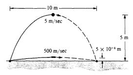
B. Tracks of ball and bullet through space as seen in laboratory have very different curvatures.
