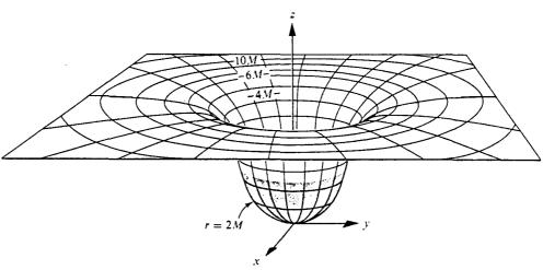
Figure 23.1. Geometry within (grey) and around (white) a star of radius R = 2.66M, schematically displayed. The star is in hydrostatic equilibrium and has zero angular momentum (spherical symmetry). The two-dimensional geometry
