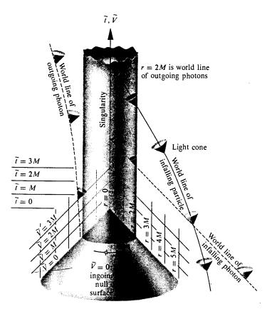
Ingoing Eddington-Finkelstein coordinates (one rotational degree of freedom is suppressed; i.e.,  $\theta$  is set equal to  $\pi/2$ ). Surfaces of constant  $\widetilde{V}$ , being ingoing null surfaces, are plotted on a 45-degree slant, just as they would be in flat spacetime. Equivalently, surfaces of constant
