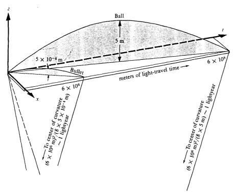
C. Tracks of ball and bullet through spacetime, as recorded in laboratory, have comparable curvatures. Track compared to arc of circle: (radius) = (horizontal distance)<sup>2</sup>/8 (rise).
