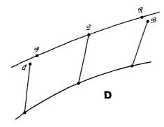
Confrontation between actual course of tracer point on test geodesic and "canonical course": course it would have had to take to keep constant separation from the tracer point moving along the fiducial geodesic.
