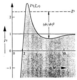
"Turning points" of orbit occur where horizontal line of height  $\widetilde{E}^2$  crosses  $\widetilde{V}^2$
