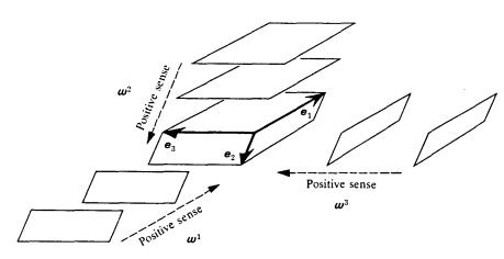
Figure 9.2. The basis vectors  $\mathbf{e}_{\alpha}$  and dual basis 1-forms  $\mathbf{w}^{\beta}$  in the tangent space of an event  $\mathscr{P}_{\mathbf{0}}$ . The condition  $\langle \mathbf{w}^{\beta}, \mathbf{e}_{\alpha} \rangle = \delta^{\beta}_{\alpha}$
