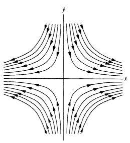
(a) Force lines for  $\ddot{A}_{\times} = 0$ ,  $\ddot{A}_{+} > 0$
