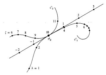
Figure 2.2. Same tangent vector derived from two very different curves. That parametrized straight line is also drawn which best fits the two curves at  $\mathcal{P}_0$ . The tangent vector reaches from 0 to 1 on this straight line.
