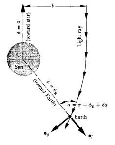
Figure 40.2. Coordinates used in the text for calculating the deflection of light. Notice that in this diagram of increases in the clockwise direction.
