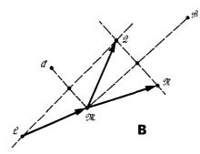
Parallel transport of  $\mathfrak{M} \mathcal{Q}$  by "Schild's ladder construction" (Box 10.2) to  $\mathfrak{M} \mathcal{B}$  and  $\mathcal{L} \mathcal{Q}$ . If the test geodesic  $n+\Delta n$  had kept a constant separation from the fiducial geodesic n, its tracer point would have arrived at  $\mathcal{Q}$  at the value  $(\lambda-\Delta\lambda)$  of the affine parameter, and at  $\mathcal{B}$  at  $(\lambda+\Delta\lambda)$ .
