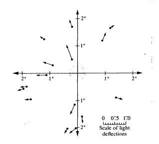
Observed light deflections (mean of two instruments) of the 15 best measured stars within 2°.5 of the sun's center in the total solar eclipse of September 21, 1922 at Wallal, Western Australia, as determined by Campbell and Trumpler (1928). The arrows represent in size and direction the observed light deflections relative to the reference stars (5° to 10° from the sun's center). (See Box 1.6 for Einstein's description of the deflection in terms of the curvature of geometry near the sun).
