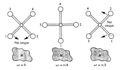
When in operation the gradiometer rotates with angular velocity  $\omega$  about its center. As it rotates, the torques on its arms oscillate:
