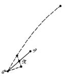
2. Take geodesic that starts at  $\mathcal{Q}$  and passes through  $\mathcal{R}$ , and extend it by an equal parameter increment to point  $\mathcal{P}$ .
