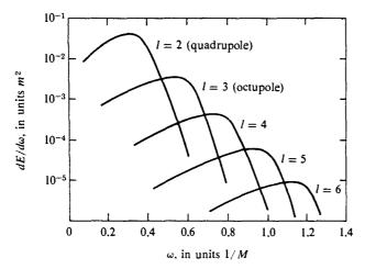
Figure 36.2. Spectrum of the gravitational waves emitted by a "delta-function" lump of matter of mass m, falling head-on into a nonrotating (Schwarzschild) black hole of mass  $M \gg m$ . The total energy radiated is distributed among multipoles according to the empirical law
